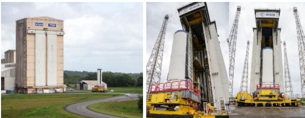
Figure 6.2.3.2.1.a – Transfer of P120C first stage atop its pallet from the Booster Integration Facility by mean of a low-slung transporter vehicle up to the mobile gantry / launch pad
