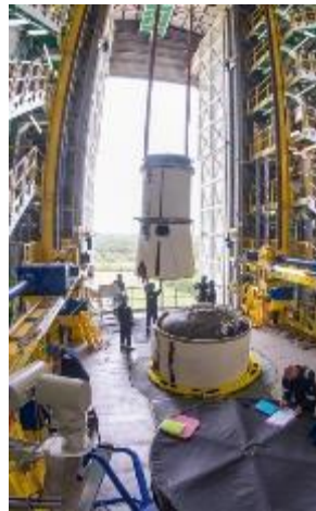
Figure 6.2.3.2.1.f – Integration on the Z9 third stage
