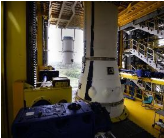
Figure 6.2.3.2.1.f – Integration on the Z9 third stage
