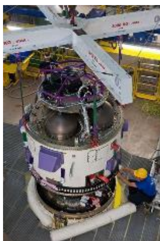
Figure 6.2.3.2.1.h – Integration of the AVUM+ upper stage
