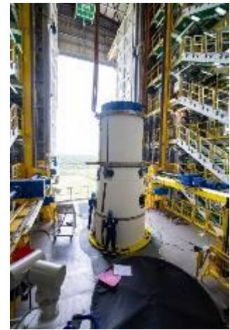
Figure 6.2.3.2.1.e – Transfer of the Z9 third stage with the 2/3 interstage up to the mobile gantry / launch pad
