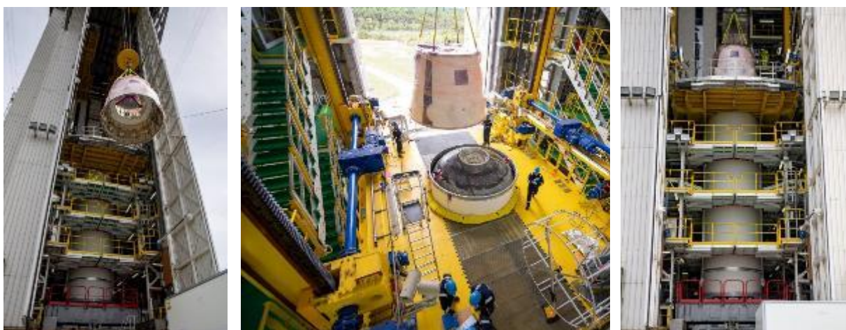
Figure 6.2.3.2.1.b – Hoisting and integration of the 1/2 interstage
