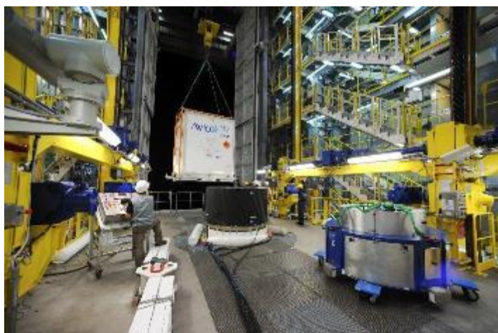
Figure 6.2.3.2.1.g – Transfer of the AVUM+ upper stage in its container and hoisting to the mobile gantry upper platform
