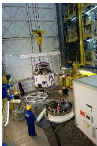
Figure 6.2.3.2.1.h – Integration of the AVUM+ upper stage
