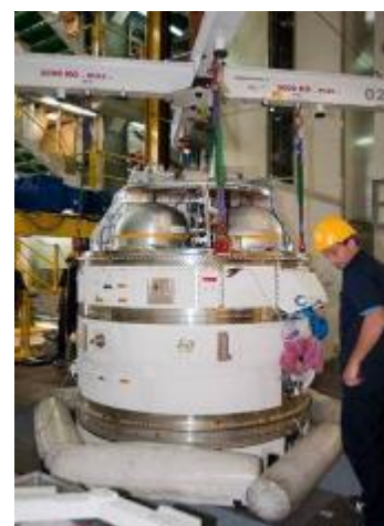
Figure 6.2.3.2.1.h – Integration of the AVUM+ upper stage
