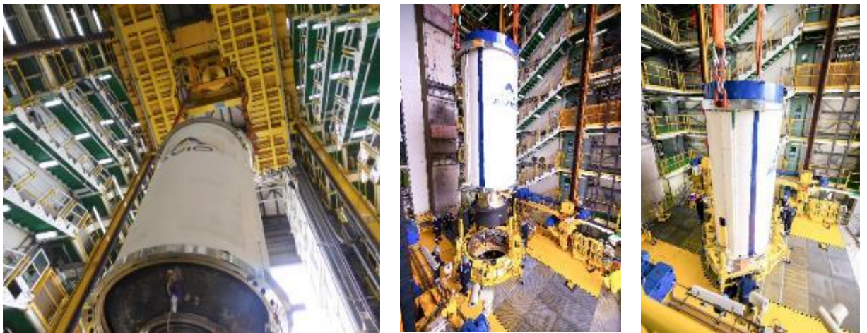
Figure 6.2.3.2.1.d – Hoisting of the Z40 second stage and integration on the 1/2 interstage
