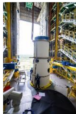
Figure 6.2.3.2.1.e – Transfer of the Z9 third stage with the 2/3 interstage up to the mobile gantry / launch pad
