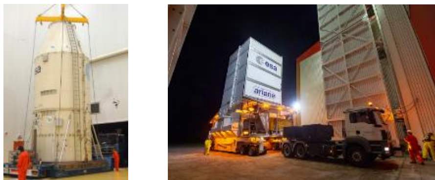
Figure 6.3.4.1.a – The CCU2 and CCU3 payload containers (for spacecraft transportation between facilities whenever necessary)
