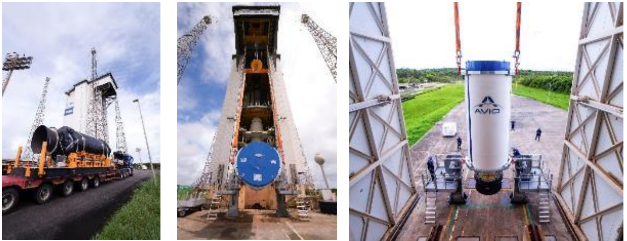
Figure 6.2.3.2.1.c – Transfer of the Z40 second stage from storage up to the mobile gantry / launch pad
