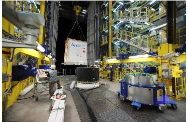
Figure 6.2.3.2.1.g – Transfer of the AVUM+ upper stage in its container and hoisting to the mobile gantry upper platform
