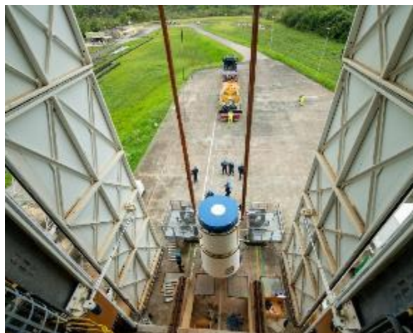
Figure 6.2.3.2.1.e – Transfer of the Z9 third stage with the 2/3 interstage up to the mobile gantry / launch pad
