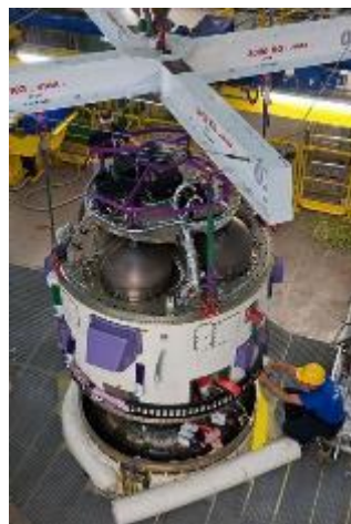
Figure 6.2.3.2.1.h – Integration of the AVUM+ upper stage
