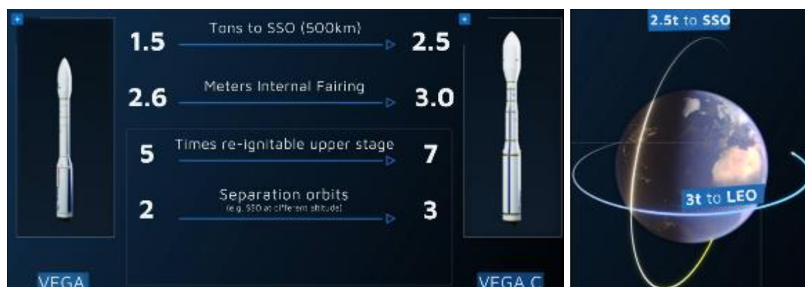
Figure 1.3.a – Evolution from Vega to Vega C
