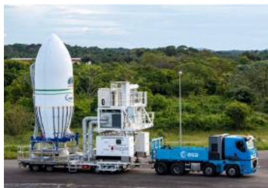
Figure 6.3.4.1.b – The PFRCS (for Payload Assembly Composite transportation to the launch pad)
