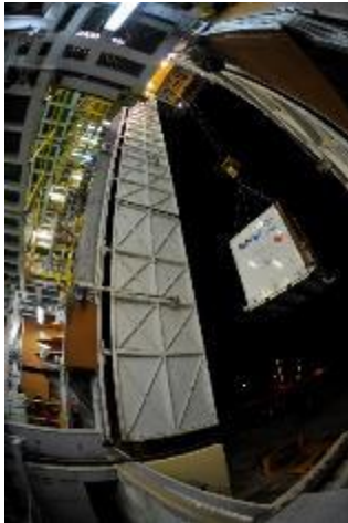
Figure 6.2.3.2.1.g – Transfer of the AVUM+ upper stage in its container and hoisting to the mobile gantry upper platform
