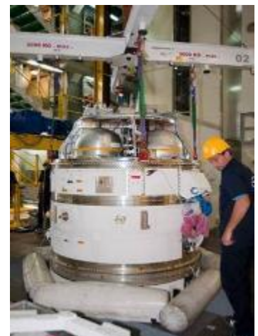
Figure 6.2.3.2.1.h – Integration of the AVUM+ upper stage
