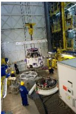
Figure 6.2.3.2.1.h – Integration of the AVUM+ upper stage
