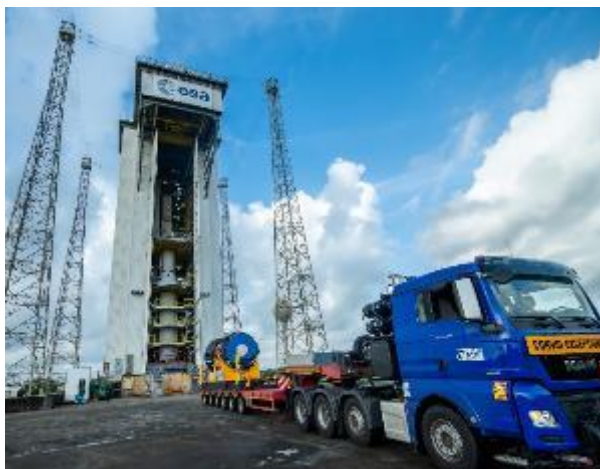
Figure 6.2.3.2.1.e – Transfer of the Z9 third stage with the 2/3 interstage up to the mobile gantry / launch pad
